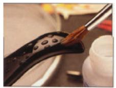
Prep the surface by brushing on a setting solution such as Microscale's Micro-Set. The solution kills any oils on the paint and forms a lubricating layer between the decal and the model.
