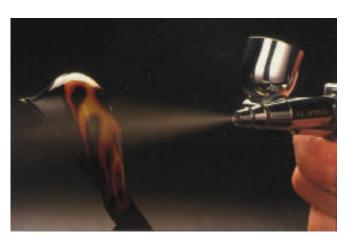
12 If the decal depicts a graphic that would be done with paint, such as these flames, it should be clearcoated to protect the decal and to give it the same shine as the painted fender.
