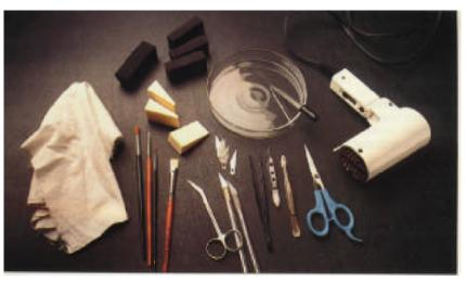
Here are the tools needed for decal application. The eyedropper in the petri dish is great for adding setting solution to the surface of a decal. The eyedropper can also be used to remove excess liquid.
