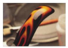
After tamping the decal in place, give it time to dry. Then, wipe it with a damp towel to remove any residue. The result should be a decal that full conforms to its surface.
