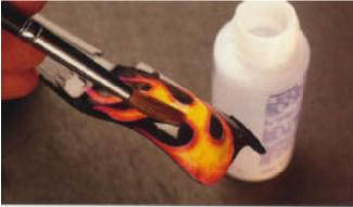
It is difficult for the decal to conform to the shape of the fenderand folds have formed at the decal's edges. It may be necessary to cut darts into the fold to allow the decal to lay flat. Several small darts are better than one big one.
